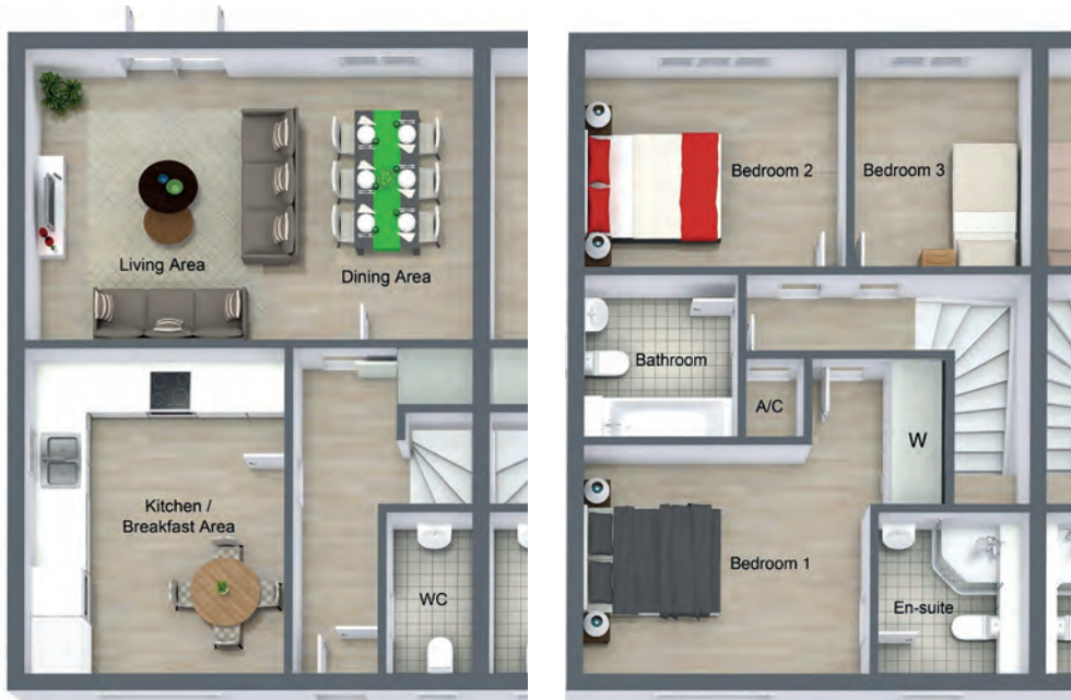
The floor plans are for plot 9, so for plot 4 are "handed"/ a mirror image.
